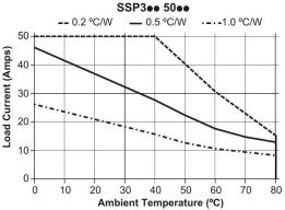
Load Current (Amps) / Courant de charge (A) / Laststrom (A) Corriente de carga (A) / Corrente di carico (Amps) / 负载电流 (A)
